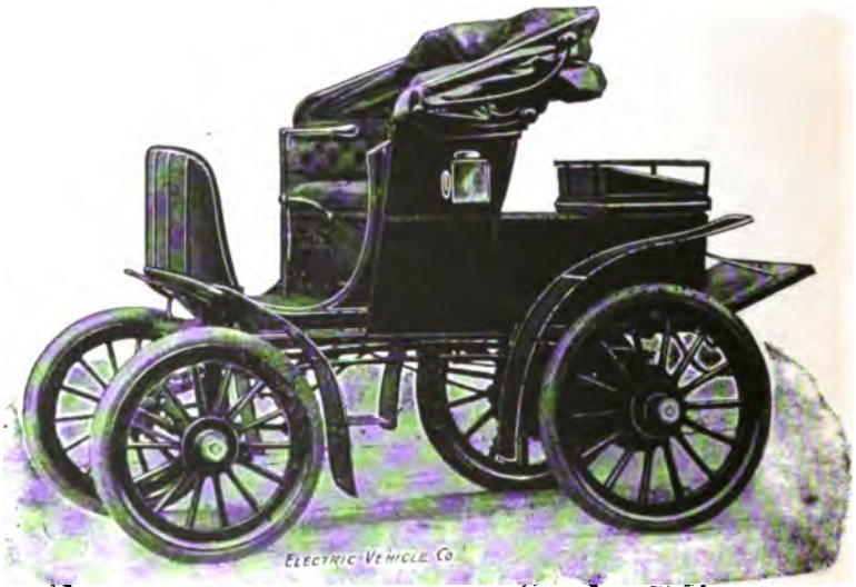
FIG. 424. —“Columbia” Electric Phaeton. This is one of the most popular and serviceable styles of American electric vehicle. It weighs about 2,800 pounds; has a radius of about forty miles per charge of battery, and a maximum speed of twelve miles per hour.
